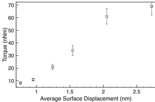
FIG. 3. Calculated maximum torque as a function of the average substrate SAW displacement for the disk with a  $50 \mu\text{l}$  water coupling layer. The torque increases substantially until the disk begins to precess at around 2.5 nm surface displacement. The error bars appear from the error in measuring angular velocity as shown in the data taken and plotted in Fig. 2.
