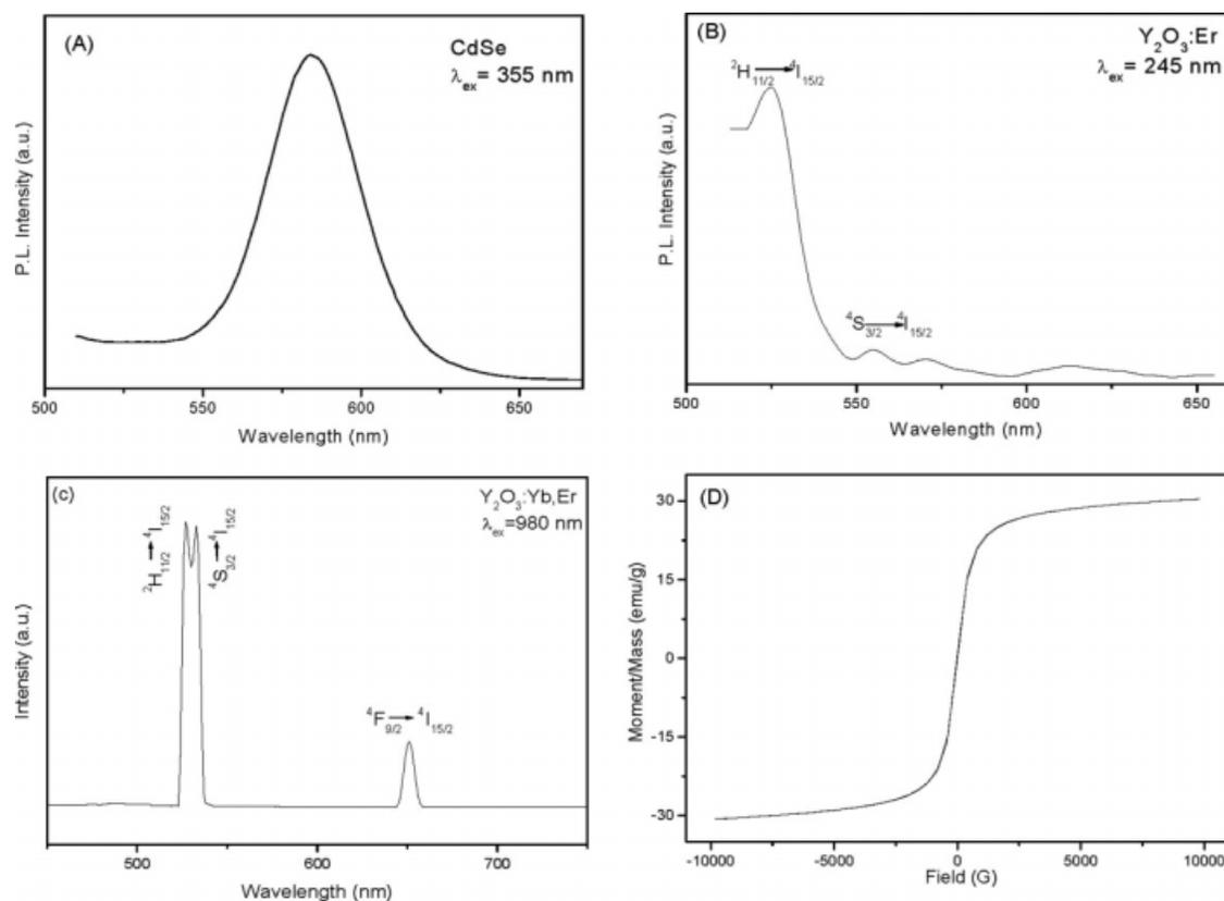
**Figure 1.** Photoluminescence spectra of (A) CdSe QDs, (B)  $Y_2O_3:Er$ , (C)  $Y_2O_3:Yb,Er$ , and (D) magnetization curve of  $\gamma-Fe_2O_3$ .
